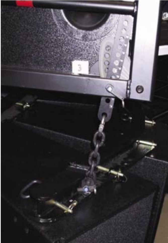
Figure 46. Pinning front adjustable link plate
